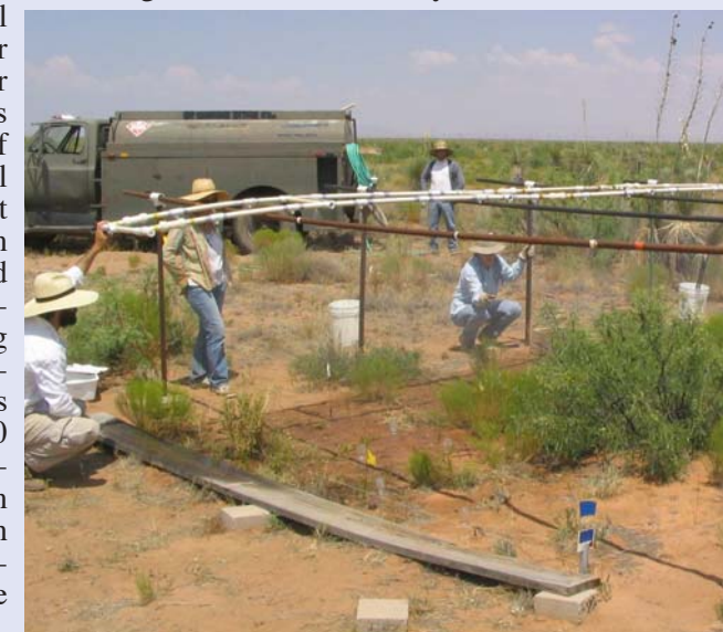
Monthly rainfall applied using a portable rainfall simulator.
